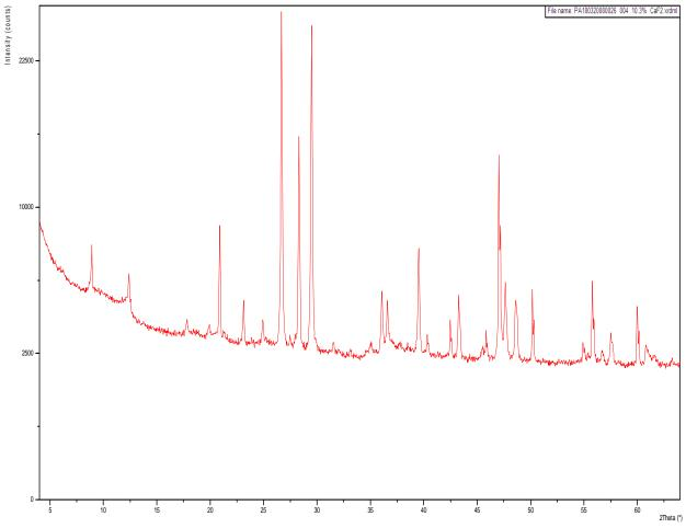
Figure 4 –X-ray diffraction pattern of the sample labeled "22C1", with degrees 2 $\theta$  along the x-axis and intensity (counts) along the y-axis.
