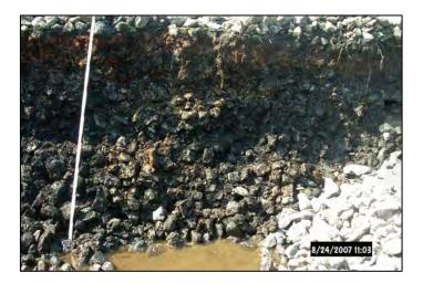
Figure 3. Manganese material filled void spaces and coated limestone aggregate prior to recovery
