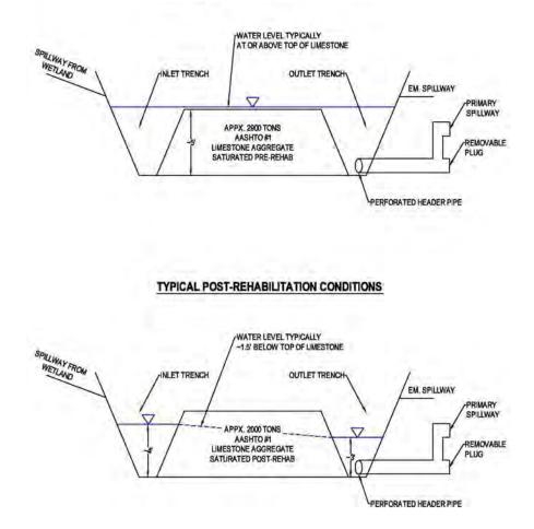
Figure 7. Typical Pre- and Post-Rehabilitation Conditions of the HFLB
