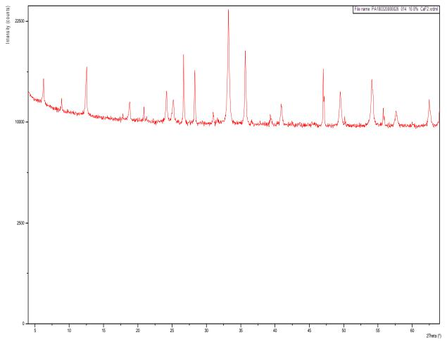
Figure 14 –X-ray diffraction pattern of the sample labeled "COM5A", with degrees 2 $\theta$  along the x-axis and intensity (counts) along the y-axis.
