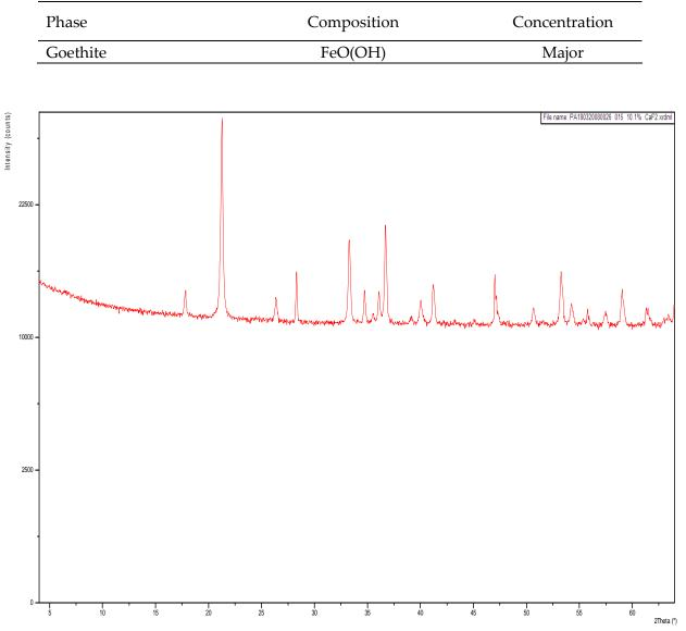
Figure 15 –X-ray diffraction pattern of the sample labeled "COM6A", with degrees  $2\theta$  along the x-axis and intensity (counts) along the y-axis.
