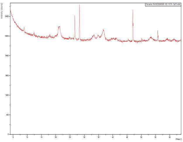
Figure 12 –X-ray diffraction pattern of the sample labeled "DS2FE2", with degrees 2θ along the x-axis and intensity (counts) along the y-axis.
