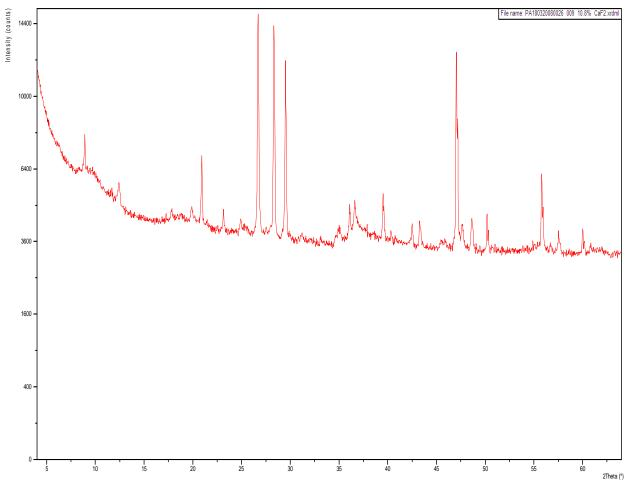
Figure 9 –X-ray diffraction pattern of the sample labeled "28A1", with degrees 2θ along the x-axis and intensity (counts) along the y-axis.
