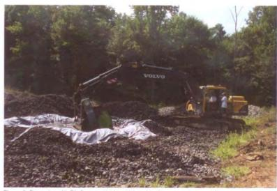
Figure 2. Excavator with FlipScreen attachment "washing" manganese covered limestone.
