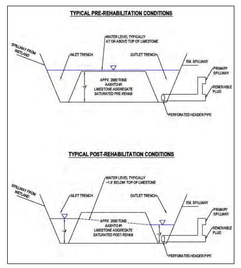
Figure 1: Comparison of Pre- and Post- Rehabilitation HFLB Conditions
