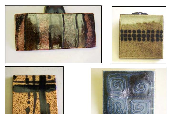
**Recovered Mn and low-pH Iron for "Green" Ceramic Tiles:** As there is a growing demand for "Green" building materials, it was only natural to pursue creating ceramic tiles made utilizing glazes containing the recovered manganese and low-pH iron. Bob Isenberg made these test/marketing pieces as examples when talking to tile manufacturers
