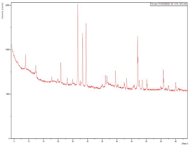
Figure 2 –X-ray diffraction pattern of the sample labeled "MN2", with degrees 2θ along the x-axis and intensity (counts) along the y-axis.
