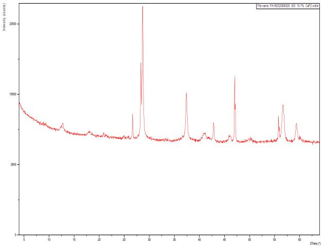
Figure 3 –X-ray diffraction pattern of the sample labeled "COM1A", with degrees 2θ along the x-axis and intensity (counts) along the y-axis.
