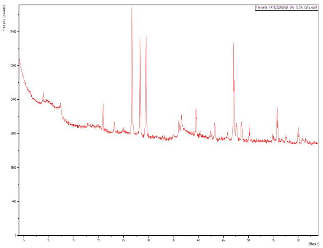
Figure 5 –X-ray diffraction pattern of the sample labeled "25A1", with degrees 2 $\theta$  along the x-axis and intensity (counts) along the y-axis.
