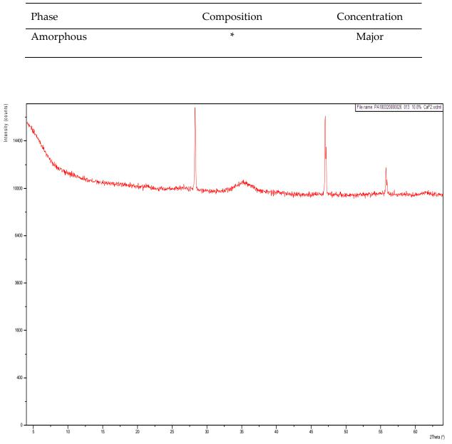
Figure 13 –X-ray diffraction pattern of the sample labeled "DS1FE1", with degrees 2 $\theta$  along the x-axis and intensity (counts) along the y-axis. The peaks at 28.3°, 47.0°, and 55.8° are from the CaF<sub>2</sub> internal standard.
