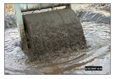
Figure 5. Close up of FlipScreen during manganese recovery operation
